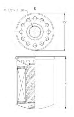
Operating Pressure: Operating Temp: Collapse Rating: Thread Size: Filtration Rating: Seal Materials 174 PSI -45° F to 255° F 116.03 psid 1-1/2″ -16 UN B<sub>1</sub> = 200 Buna Gasket
