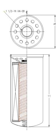
$\begin{array}{lll} \mbox{Operating Pressure:} & 100 \mbox{ PSI} \\ \mbox{Operating Temp:} & -40^{\circ}\mbox{F to } 225^{\circ}\mbox{F} \\ \mbox{Collapse Rating:} & 80 \mbox{ PSID} \\ \mbox{Thread Size:} & 1-1/2" - 16 \mbox{ UNF} \\ \mbox{Filtration Rating:} & \mbox{B}_3 = 200 \end{array}$
