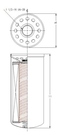
Operating Pressure: 100 PSI Operating Temp:  $-40^{\circ}\text{F}$  to 225°F Collapse Rating: 80 PSID Thread Size: 1-1/2" - 16 UNF Filtration Rating:  $B_3 = 200$
