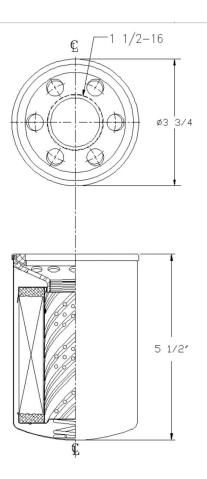
**Operating Pressure:** 225 PSI -65° F to 250° F **Operating Temp:** Collapse Rating: **80 PSID MAX** Thread Size: 1 1/2-16 Filtration Rating:  $B_1 = 200$ Seal Materials: **Buna Gasket** Gasket ID: 2-21/32" 3-15/32" Gasket OD:
